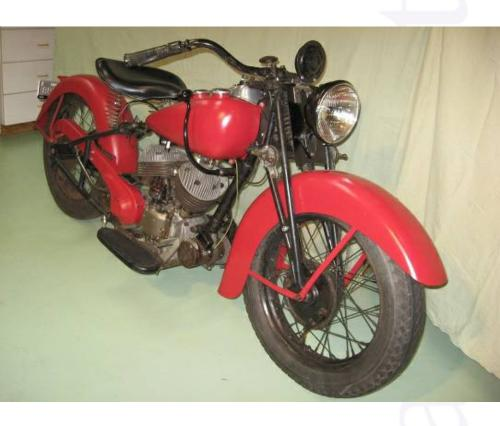
1940 Indian Sport Scout Motorcycle. It is fairly complete restoration project with a real nice frame, fenders, front fork, and handlebar assembly. These bikes have a 750cc (45 cubic inch) flathead v-twin motor that has good power to weight ratio and is fun to ride. The open fendered early post war Indians are
